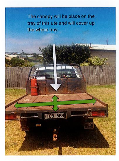
The canopy will be bolted to the tray through 4 bolts which will go through the floor and into the tray.
