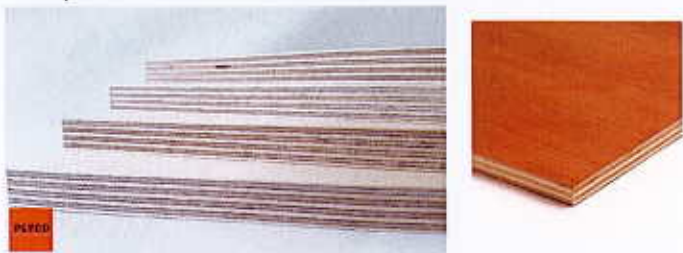
An example of the two material. High grade plywood on the left and low grade plywood with a veneer on the right.
